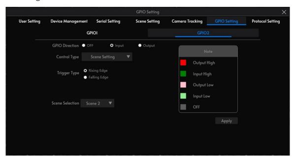
The PC enters the GPIO-2 control window, selects the [Input] direction, the control type [Scene Setting], the trigger type [Rising Edge], the parameter settings are loaded to [Scene 2], and clicks the [Apply] button at the bottom of the window.
