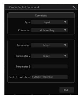
The Central Command Generator is able to convert frequently used operations into a 16-character command code for easy invocation by external devices.
