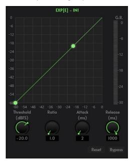
Threshold (-60 ~ 20): Sets the point from which the attenuation is calculated based on the Ratio setting. This is where the Expander starts working. When the input signal falls below the Threshold Level, the Expander compresses the signal at a preset Ratio to increase its dynamic range. When the input signal exceeds the Threshold Level, the signal is output at a 1:1 Ratio, preserving its original dynamic range. The Threshold setting requires adjustment based on the specific application scenario;
