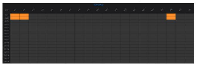
The signals of input channels IN1 and IN2 will be processed for ANS and output in output channels OUT1 and OUT2, configured as shown in the figure above:
