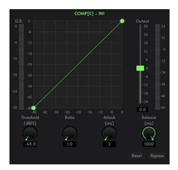
1) Threshold (-48~0): Sets the level where compression begins. This is the point from which the amount of attenuation is calculated based on the Ratio setting. A level below the Threshold Level is not compressed, anything above the Threshold Level attenuation is applied;
