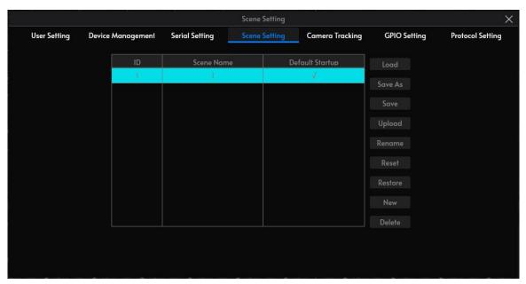
1 **Load Scene:** Load a saved scene file and restore the scene parameters to their last saved state. After the user selects the target scene file in the scene list interface, clicking the
