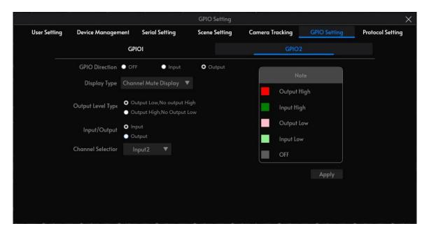
The PC enters the GPIO-2 control window, selects [Output] mode, display type [Channel Mute Display], trigger type [Output Low, No Output High], parameter setting [Inputs] channel selection [Input 2], and clicks the [Apply] button at the bottom of the window.
