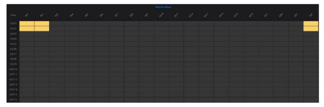
For example, the signals of input channels IN1 and IN2 are automatically mixed and output in output channels OUT1 and OUT2, as shown in the figure above:
