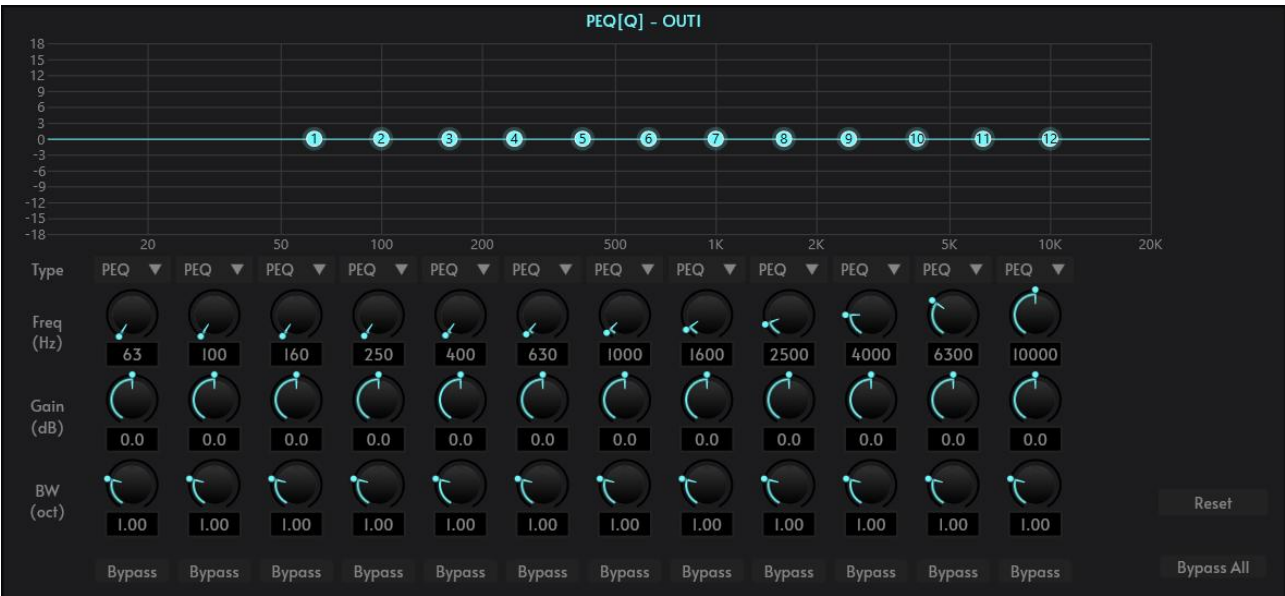
Reference Input Component Configuration - Parametric Equalizer.
