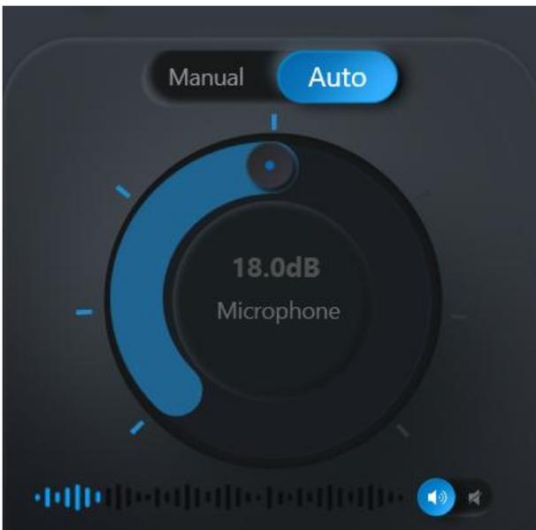
**Auto Level:** In Auto Level mode, the microphone gain is automatically adjusted by the device according to the external sound level. That is, when the external sound is loud, the device will adjust the microphone gain down; when the external sound is small, the device will adjust the microphone gain up (the microphone gain adjustment control is disabled in this mode).
