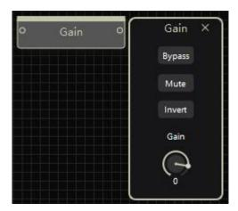
The number of signal pins is variable and set in the component's Channel number Property.
