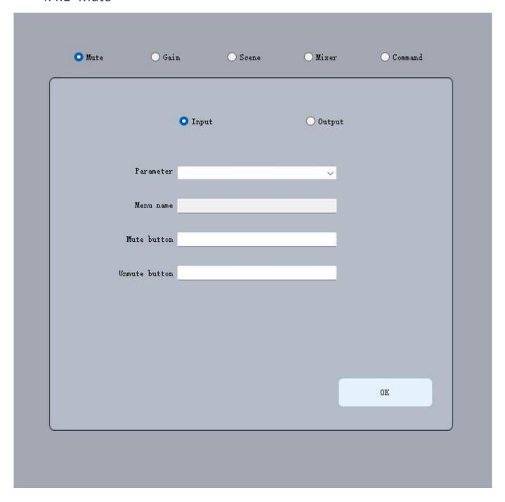
Users can select input or output parameters, display the corresponding menu name, and also customize the mute and unmute identifiers with different characters to achieve control of the processor mute state.
