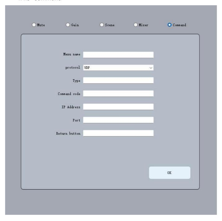
Users can customize the menu name, command type and return button with different characters, the correct central command code, IP address and port number, to achieve the control of the corresponding IP and port devices.
