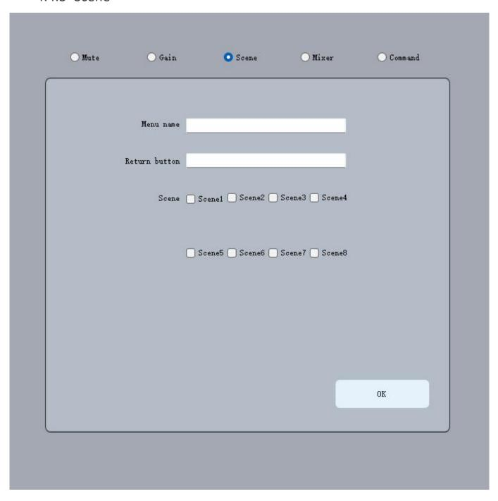
Users can customize the menu name and back button with different characters, and can also check the scenes that the processor can load to achieve control of the processor to switch scenes.
