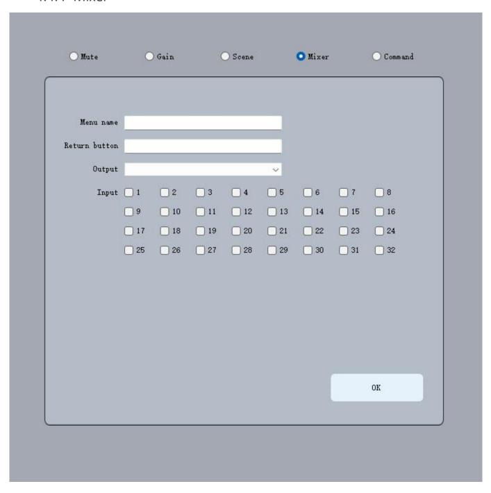
Users can customize the menu name and return button with different characters, and also select the processor output parameters as well as check the input parameters to control the processor input and output channels.
