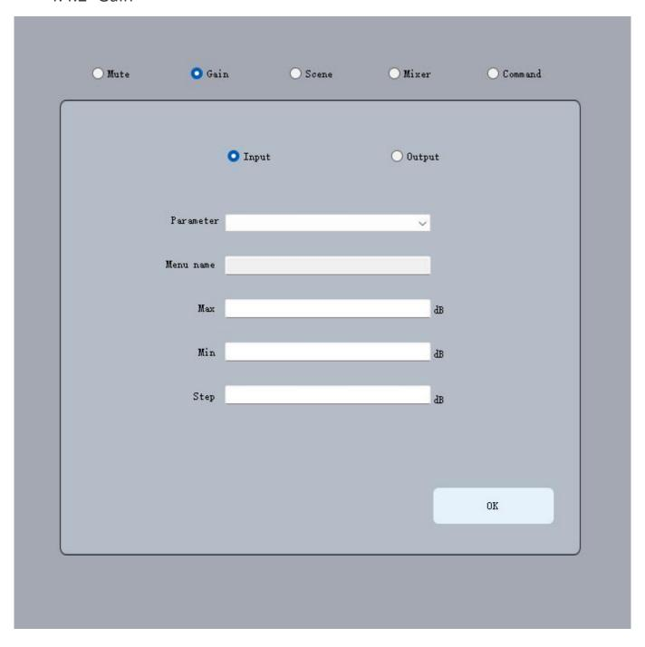
Users can select input or output parameters, display the corresponding menu name, and also set the maximum value, minimum value and step size of the processor gain (the maximum value is 12, the minimum value is -72, and the step size is  $\geq$  0.1) to achieve the control of the processor gain value.
