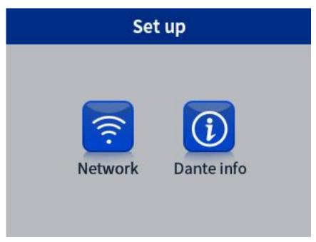
Network: For manually configuring or automatically obtaining network IP addresses; Dante info:For viewing Dante configuration information.
