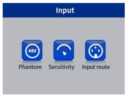
Phantom: For providing 48V voltage to condenser microphones;
