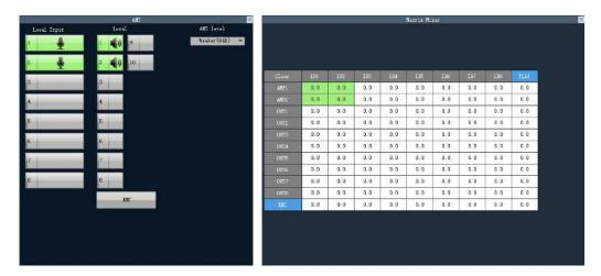
The local input IN1 and IN2 channel signals are processed for ANS and output on OUT1 and OUT2 channels, configured as above:
