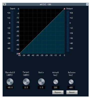
1 Threshold (-60~0): The level at which the AGC Component becomes active. This should be set at a level so that the anticipated background noise does not activate the AGC. When an Input exceeds the Threshold Level, the Gain for that input is adjusted to calculated level based on the Ratio and the Target Level;
