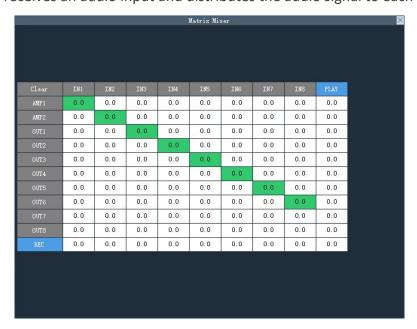
Matrix both signal routing and mixing double multiplexing function, X-axis is the input channel, Y-axis is the output channel, the matrix initialization state is (as shown in the figure above: one-to-one) input and output.
