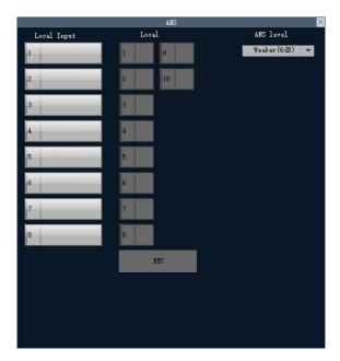
Adaptive Noise Suppression: Select the signal that needs Adaptive Noise Suppression processing, and the processed signal is output in the mixer by selecting the corresponding channel;
