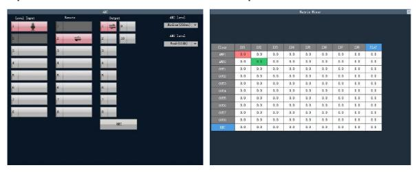
The local input signal is IN1 channel and the remote input signal is IN2 channel, at this time, the local input and the corresponding channel of the remote input will be grayed out to prevent the AEC from being activated abnormally due to the checking, and the local input signal will be AEC from OUT1 channel to the remote place, and the configuration will be as described in the above figure:
