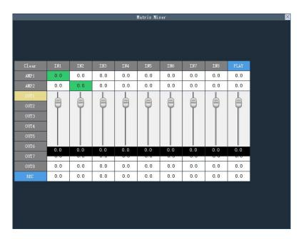
The OUT channel of the mixer is equipped with a gain fader, which allows you to individually control the gain of any output channel with a gain range of (12~-72dB).
