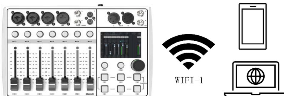
The device needs to be connected to the public WIFI network, for example, the current public WIFI network is WIFI-1, and the mobile phone、computer and mixer device should be connected to WIFI-1, making the network of all devices in the same network
