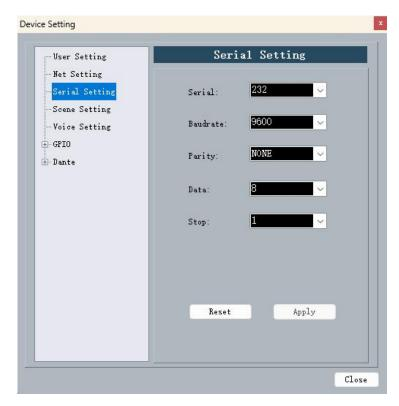
Serial window can view or modify the RS232/RS485 serial port number baud rate, check bit, data bit, stop bit settings are complete, click on the [Apply] button to modify the current device's serial port information, such as the need to restore to the initial default value, click on the [Reset] button, you can restore the settings of the parameter can not be empty.
