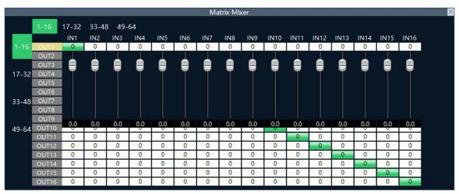
The OUT channel of the mixer is equipped with a gain fader, which allows you to individually control the gain of any output channel with a gain range of (12~-72dB).
