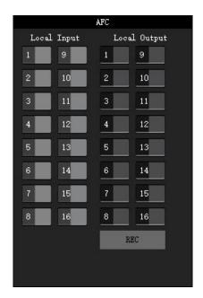
Feedback: Selects the signal that needs to be processed by the Acoustic Feedback Canceler, and the processed signal selects the output channel in the mixer;
