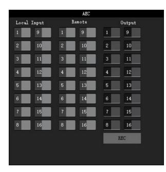
Acoustic Echo Canceler: Set the signal that needs to be processed by the Acoustic Echo Canceler, and the processed signal selects the output channel in the Mixer;
