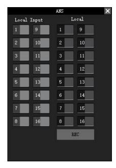
Adaptive Noise Suppression: Select the signal that needs Adaptive Noise Suppression processing, and the processed signal is output in the mixer by selecting the corresponding channel;
