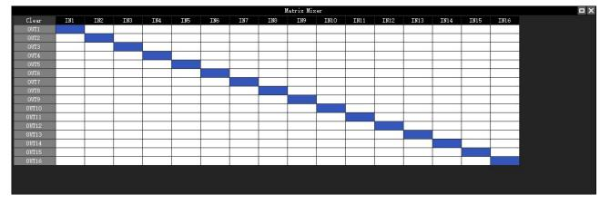
Matrix both signal routing and mixing double multiplexing function, the control logic is horizontal for the input channel, vertical for the output channel, the matrix initialization state is (as shown in the figure above: one-to-one) input and output.
