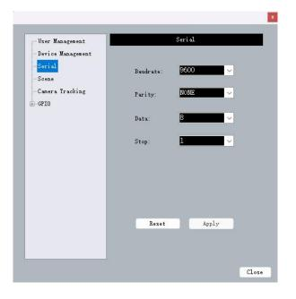
Serial window can view or modify the RS485 serial port number baud rate, check bit, data bit, stop bit settings are complete, click on the [Apply] button to modify the current device's serial port information, such as the need to restore to the initial default value, click on the [Reset] button, you can restore the settings of the parameter can not be empty.
