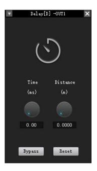
The time interval between the input of a signal to this processor and the output of this processor is generally used to produce other effects such as reverberation or echo, and can equally be used to act as a treatment for auxiliary loudspeakers in larger rendition situations.
