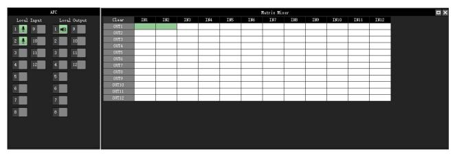
The signals from input channels IN1 and IN2 are processed in the AFC and output in output channel OUT1, configured as shown above:
